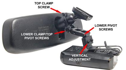
6 - Install the RD onto the mount. Make the necessary adjustments as shown above. Using the vertical adjustment and pivoting the Center Link, we recommend you adjust the RD as close to the bottom of the mirror as possible. If you are unable to get your finger between the RD and the mirror to access the top RD buttons, the spring clip is designed to be pushed downward to allow access to the top RD buttons as shown below in step 8.
