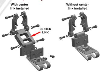
5 - The center-link may be removed if an overall shorter mount length is needed, depending on your rear view miror and desired position for the radar detector.
